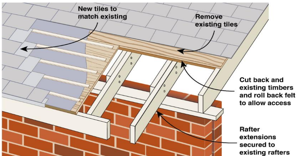
Figure 6 Eaves Roofline Extension Example
